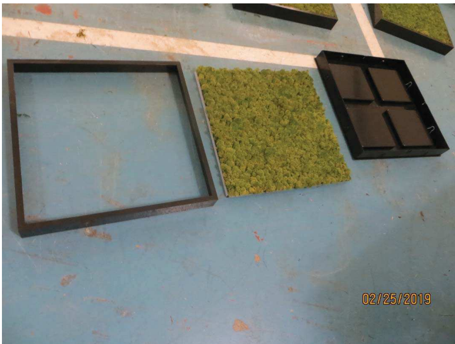
Figure 2 – Frame pieces (left, right), tray with organic material (center)
